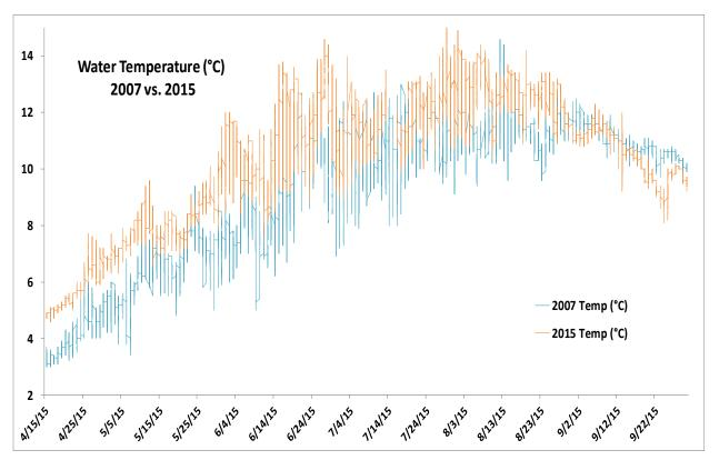
A comparison of water temperature measurements outside Homer Harbor measured every 15 minutes for the spring and summer of 2007 (blue) and 2015 (orange). Data from KBRR buoy
