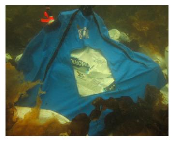
D. vex enclosure dome in place on the bottom housing the salt treatment. Above Photo: Ian Davidson. Taking Data underwater. Right Photo: Ian Davidson
