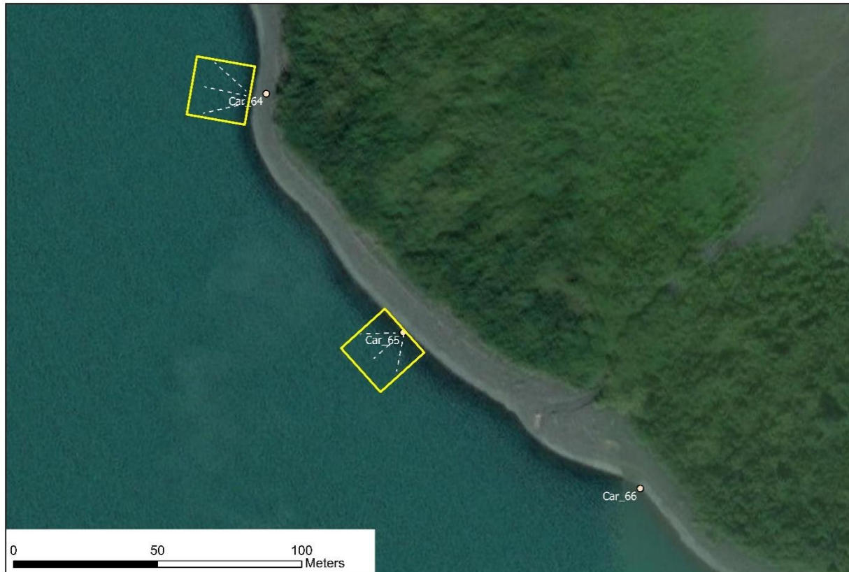
Figure 13. Example of named sampling stations. The yellow square estimates a 10 m grid to visually search for Elodea at the sample station before the rake is thrown. The white dashed lines show the directions of the rake throw.
